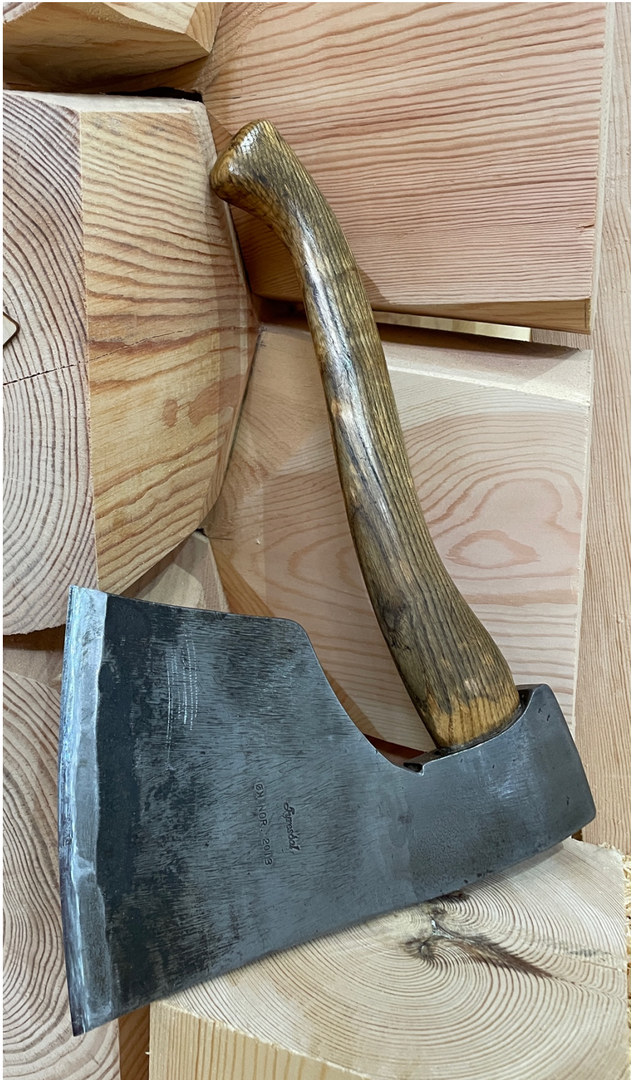
Hand-forged axe for Diamond Notch joinery Specialised hand-forged axe used for cutting Diamond Notch joints in log construction.
