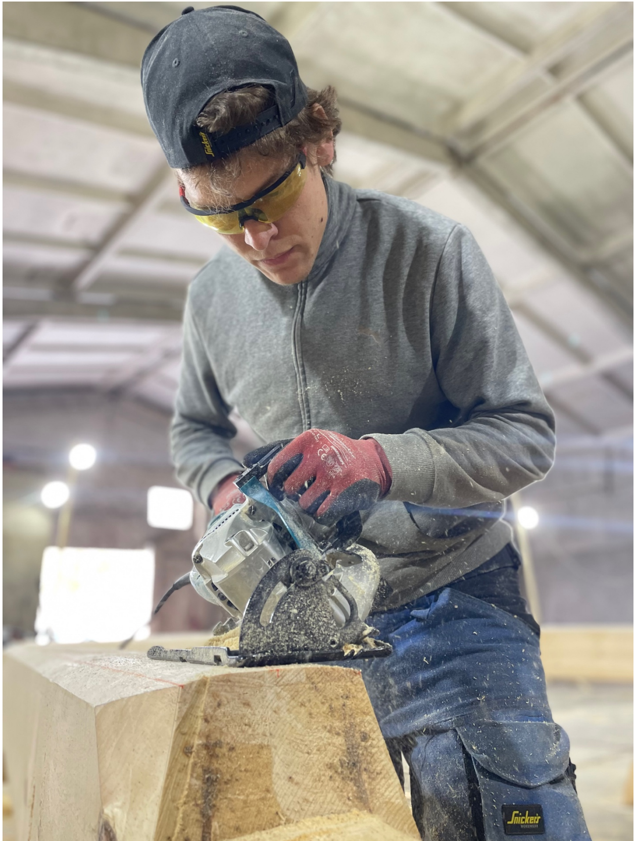
Crafting a structural timber element Process image showing the hand preparation of a structural element for a log house.
